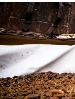
Working with local industries in al-Hasa, date palm waste is crushed into powder and added to drilling fluids to prevent the loss of circulation. This novel approach, under investigation by our R&D Center in Dhahran, could reduce costs and generate new business opportunities.
